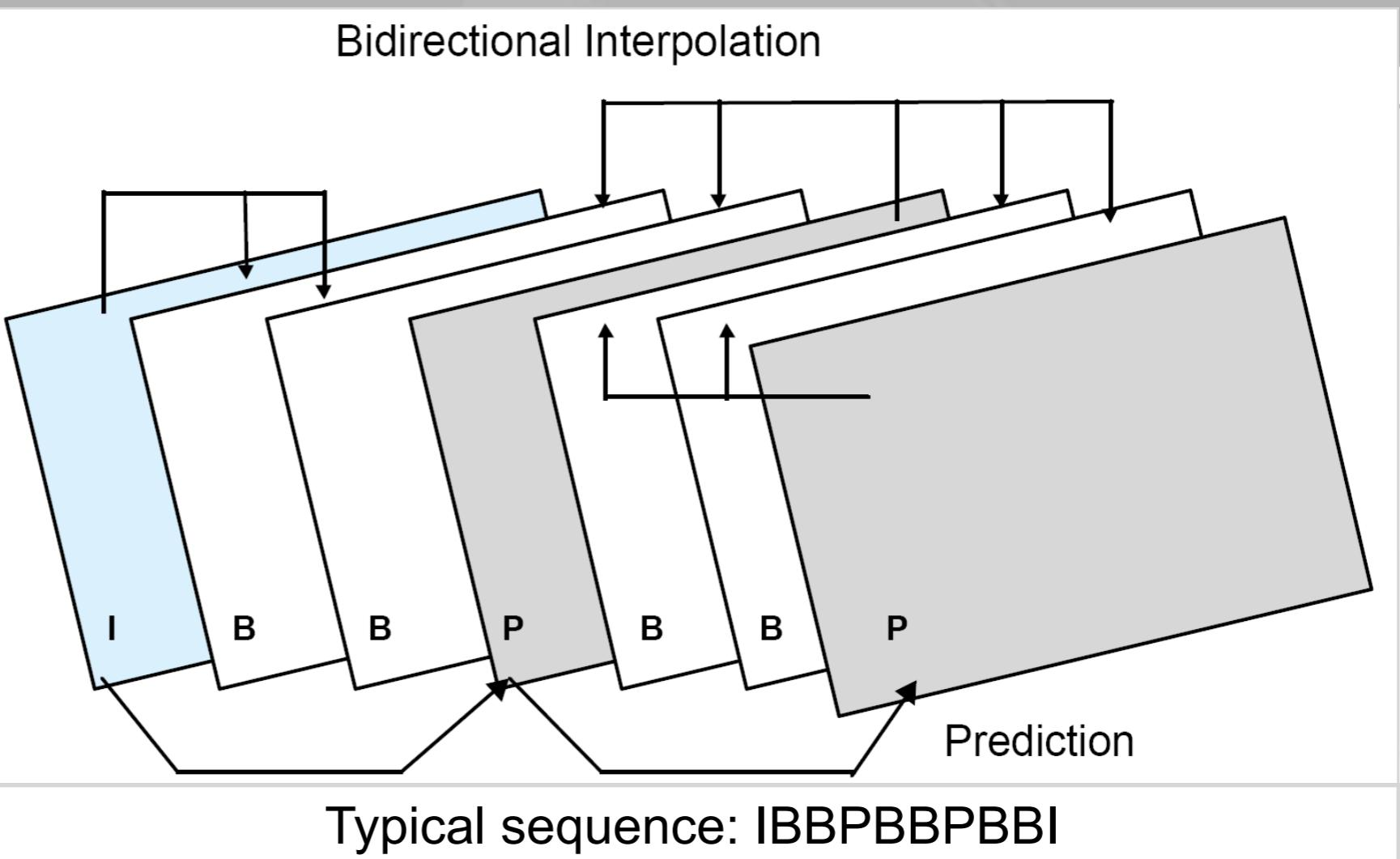
**Video signal: stream of picture, it is not necessary to send every picture**
